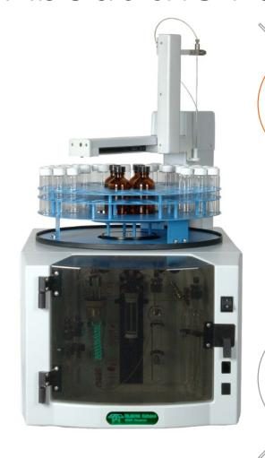
UV/Persulfate Oxidation with NDIR Detector
